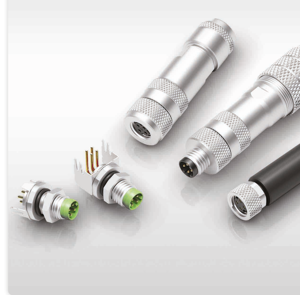
Figure 4: M8 connector with D coding and screw locking for Ethernet connectivity including power supply of Industrial IoT components. The connection meets the requirements of protection degree IP67 when mated and locked
