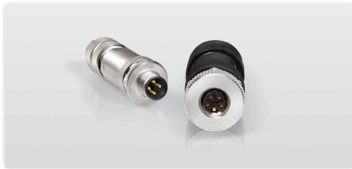
Figure 3: Contact robustness is a question of material; beryllium copper and gold plating are recommended if frequent mating is required
