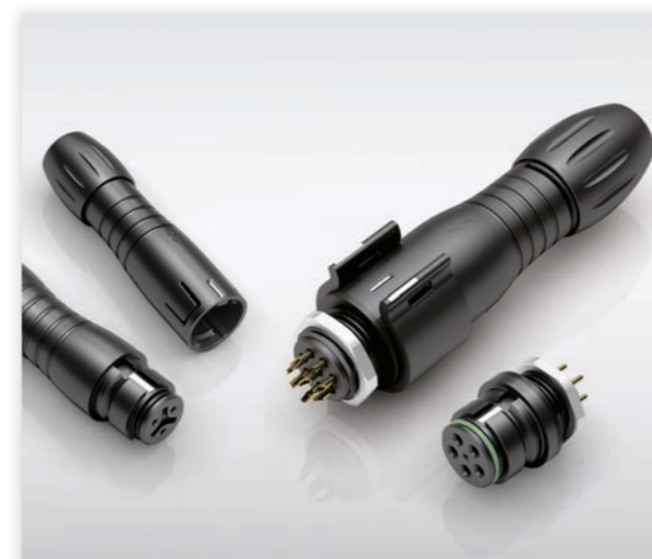
Figure 3: Miniaturized and waterproof to IP67: The 620 and 720 series with O-ring on the female side and seal in the clamping area
