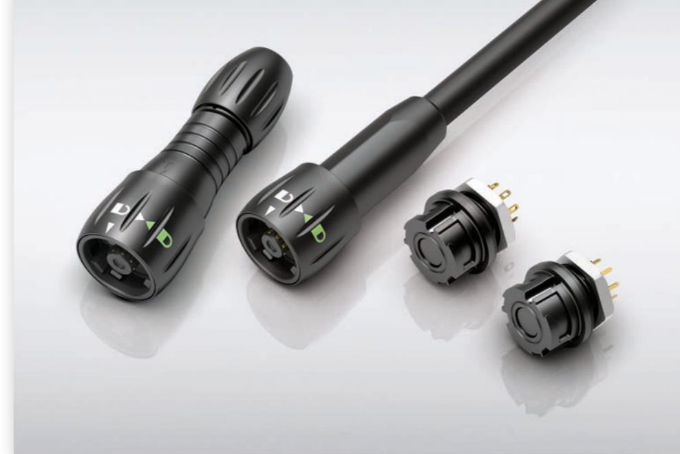
Figure 2: Not Connected Closed – thanks to a spring-loaded plastic cover, the NCC connectors of the 770 series are protected from particles and splash water even when unplugged
