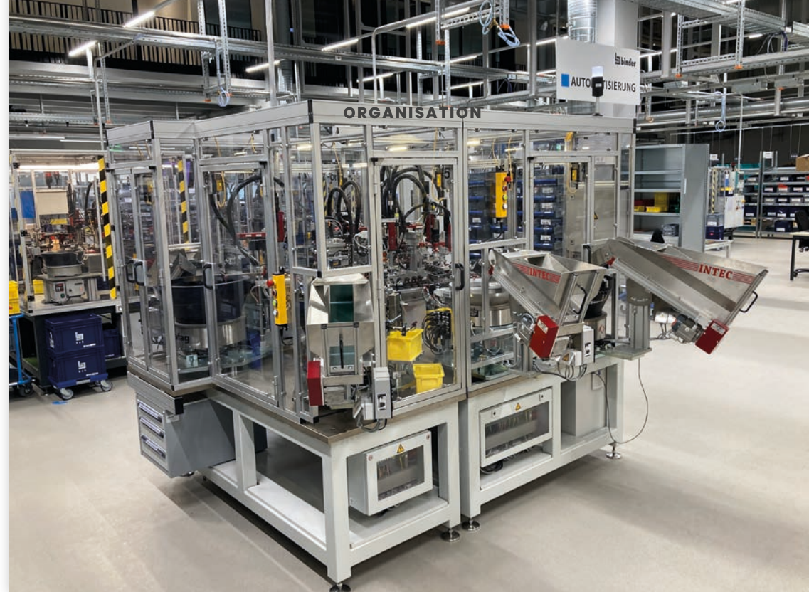
The 'PG-Twin 2' automatic screwdriver is designed for the production of 23 different coupling sleeve assemblies.
